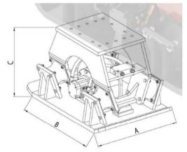
**PC Hydraulic Compactors** are mounted on Mini Excavators, Backhoe-Loaders and similar Main Machines with hydraulic power unit. Hydraulic Compactor does compacting by high frequency impact power. This vibration force is used for compacting of soil, granularmaterial, piles, driving of post and steel sheeting timber. The optional rotation functionturns the compactor 360 degree.
